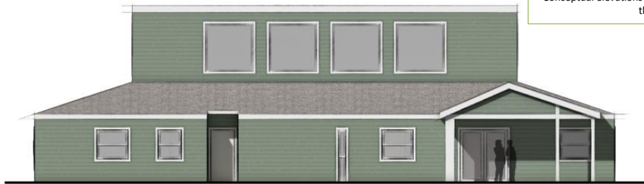
Conceptual elevations of the new front entry canopy that mimics the existing roof lines .
